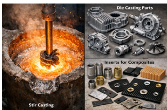
Fig 3 Stir casting process for manufacturing of composites by casting process
